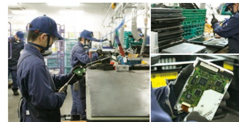
Copper is mainly recovered from A/C piping, while gold and silver are recovered from IT device circuit boards.
