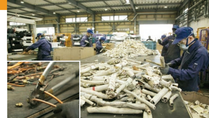
Copper is mainly recovered from A/C piping, while gold and silver are recovered from IT device circuit boards.
